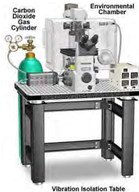
**Figure 1-7: Schematic drawing of a live imaging setup**
