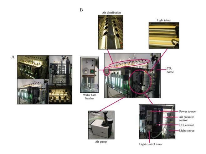
**Figure 5.** System used for the growth of  $air/CO_2$  bubbled cultures of *Anabaena* sp. PCC 7120; (A) presents the complete system and (B) presents the more important parts separately.
