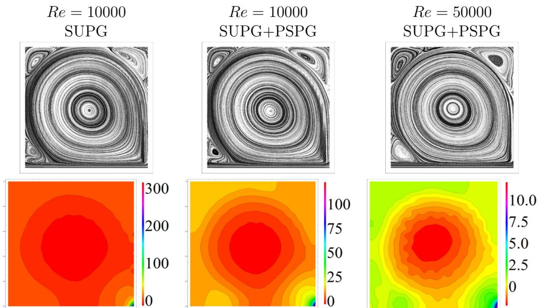
Figure 3: Stationary Navier-Stokes problem. Solution with stabilization techniques. Velocity is illustrated at the upper figures, pressure is illustrated at lower figures.
