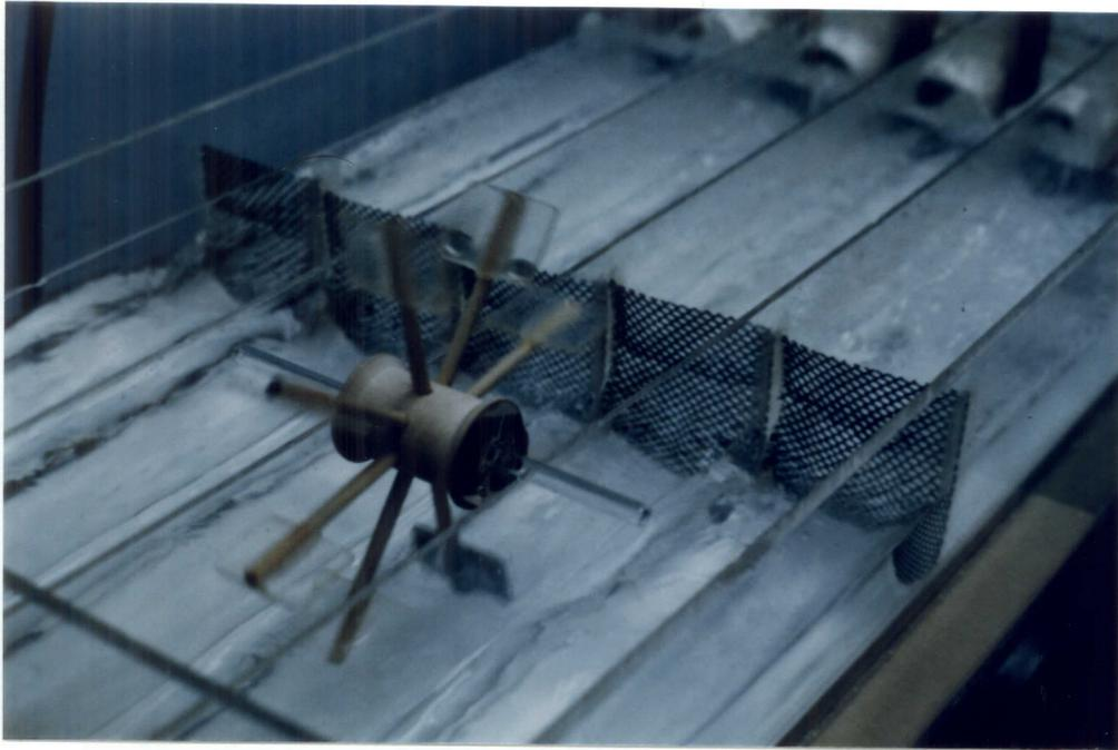
A.C. centrifugal pump moved water from a 170 l reservoir tank to the swim channels, which drained back into the tank. Water flow into channels was controlled with P.V.C. valves in the plumbing at the head of each channel. A single plexiglas vane behind the channels controlled outflow from them. Water depth in channels was maintained at 6 cm.
