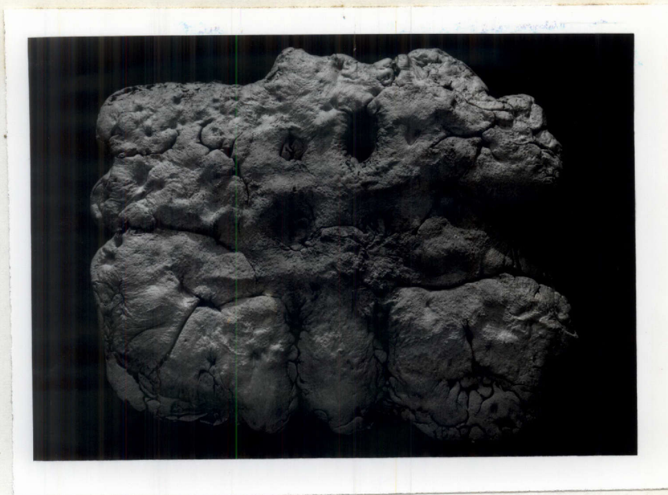
Fig. 28--Series III casting result using a melt temperature of 1503°F and only water as a binder.
