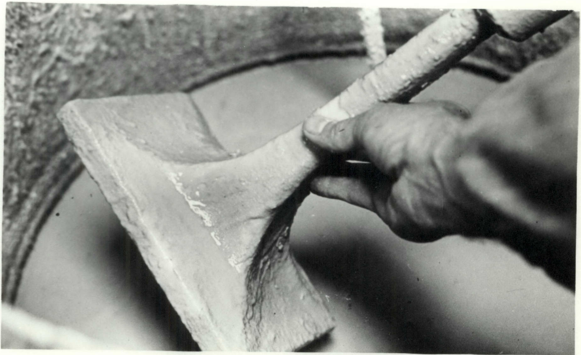
Fig. 36--Second dip-coating of pattern one
