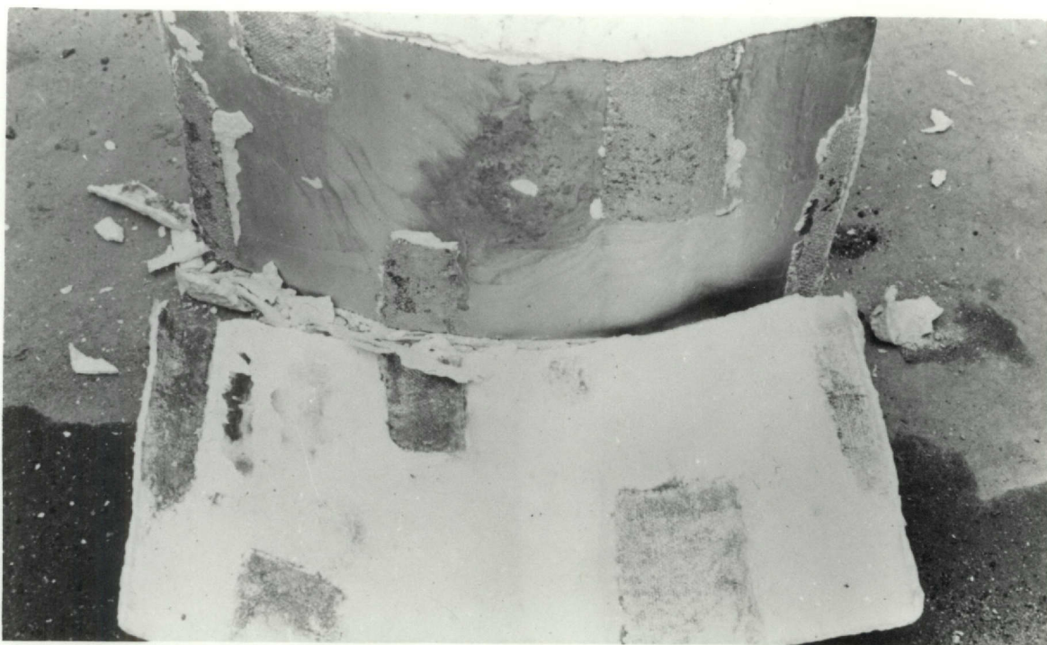
Fig. 90--Cast of pattern ten: trial 2, emerging from mold
