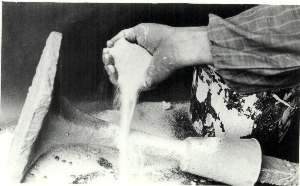
Fig. 37--Second stuccoing of pattern one
