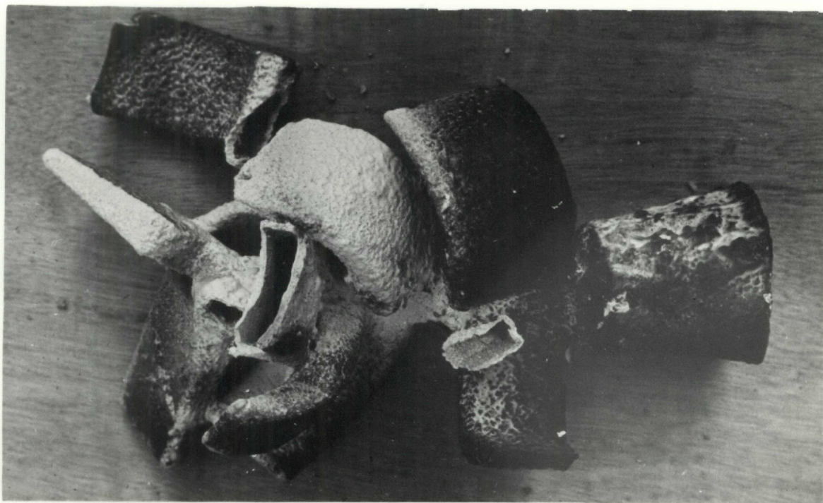
Fig. 7--Molds for Bondo (c.) finished patterns
