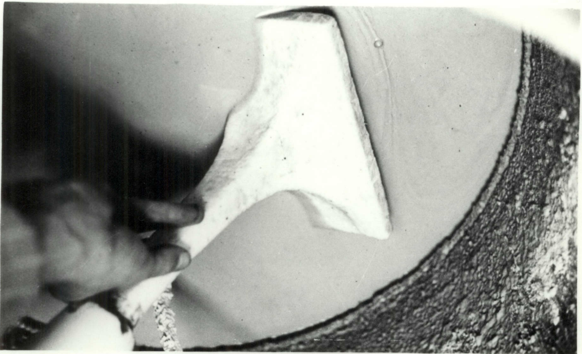
Fig. 32--First dip-coating of pattern one
