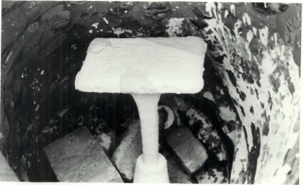
Fig. 41--Burning out pattern one
