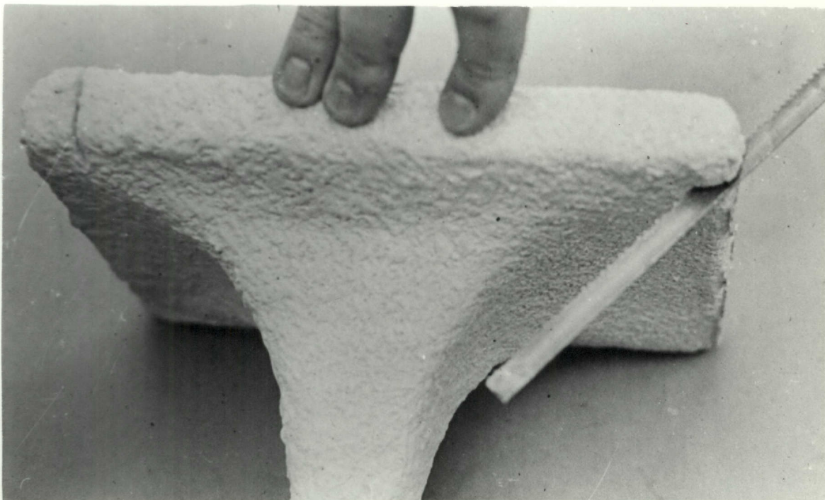
Fig. 40--Slit venting pattern one
