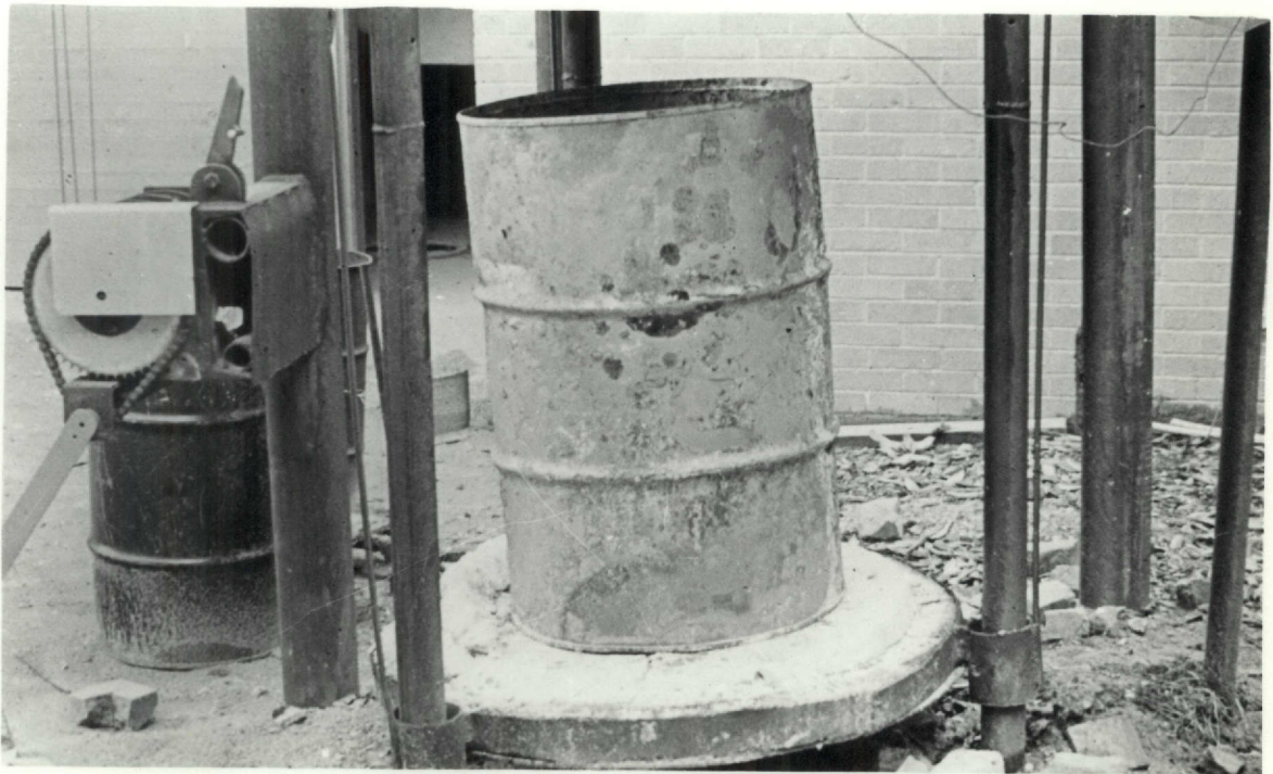
Fig. 42--Muffle for burn out
