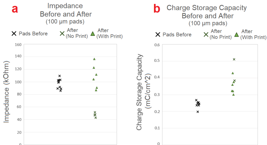
Figure 17 a) Mean impedance values from each 100 \mu\text{m} electrode pad on one wafer, before printing, sputtering, and etching process. Three measurements were taken and averaged from each pad to produce each point shown. Some pads were not printed on but still underwent the sputtering and etching process to serve as comparisons. b) Mean charge storage capacity measurements from the same set of 100 \mu\text{m} electrode pads. Two measurements were taken and averaged from each pad to produce each point shown.
