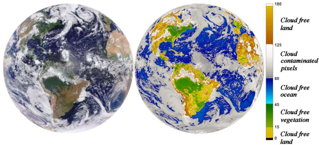
Figure 4. Left panel shows an EPIC RGB image taken on 23 August 2016 at 15:24:58 GMT. Equation (7) was applied to each image pixel. Right panel shows the distribution of ERTI over sunlit Earth. Its values corresponding to cloud-free ocean, land, vegetation, and cloudy pixels tend to occupy different spaces within the 0^\circ to 180^\circ interval. Phase angle is 5.65^\circ . Color bar shows thresholds for different reflector types.
