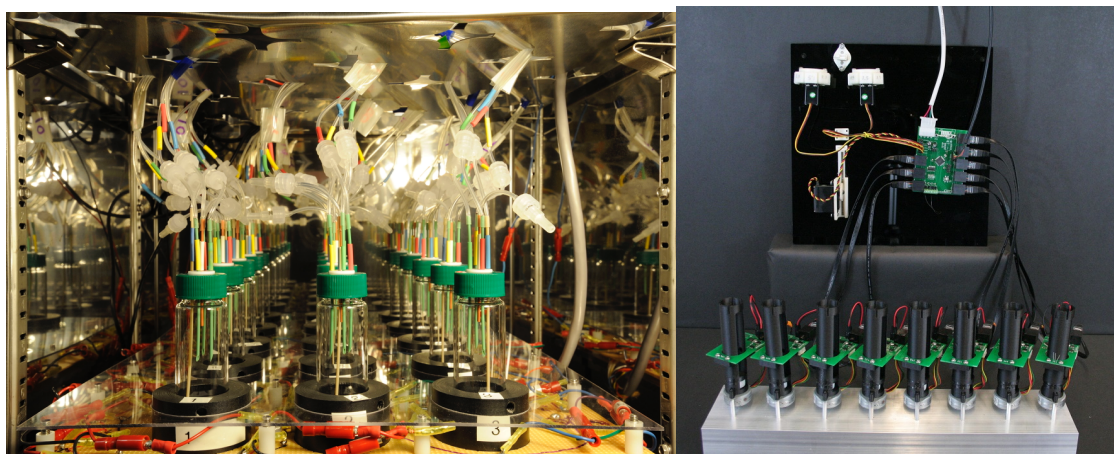
Figure 1-4: DIY Continuous Culture Systems. (left) Morbidostat system designed to study antibiotic resistance and evolution. (right) Flexostat system designed to probe synthetic circuits in more defined conditions. Each need to be housed in an incubator and electronic components used are not compatible. Reproduced from Toprak 22 and Takahashi 13 .
