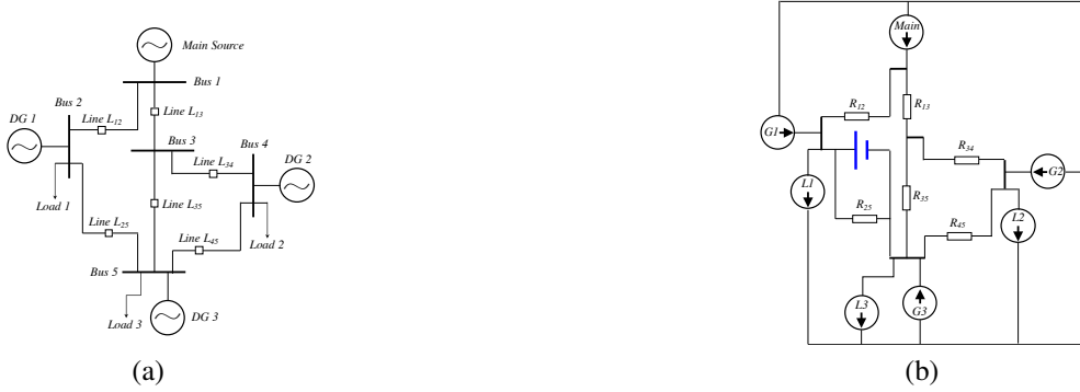
Fig. 1. (a) A 5-bus network with line overload at Line L 25 . (b) The equivalent mixed-source circuit of (a) with the voltage source (blue) denoting the effect of load regulating equipment at Bus 2 and Bus 5 .
