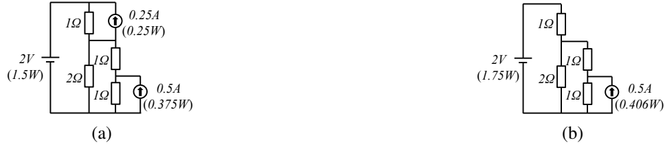
Fig. 5. (a) A mixed-source network with two current sources and one voltage source. (b) A mixed-source network with one current source and one voltage sources. (Example from [2]).
