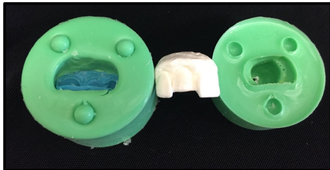
Figure 21: Cured epoxy resin abutment
