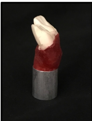
Figure 18: Epoxy resin master die fixed at 125° angle
