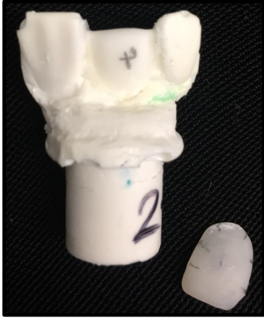
Figure 36: Mode of failure of Lava Ultimate at 0.4mm, 0.7mm and 1.0mm, Adhesive failure
