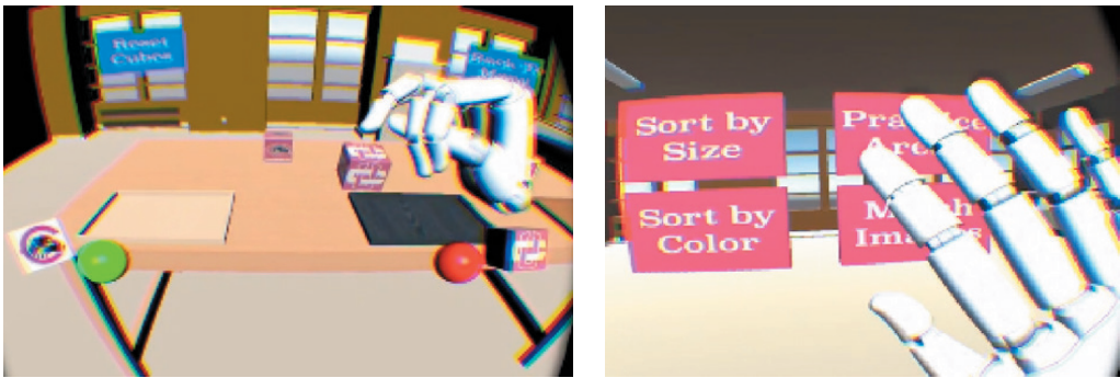
Figure 5. Visual channel filtered to highlight salient information. Left: colored balls indicate correct placement of block. Right: red squares have 4 available choices, obscuring any other activity the user might engage in beside making a choice.
