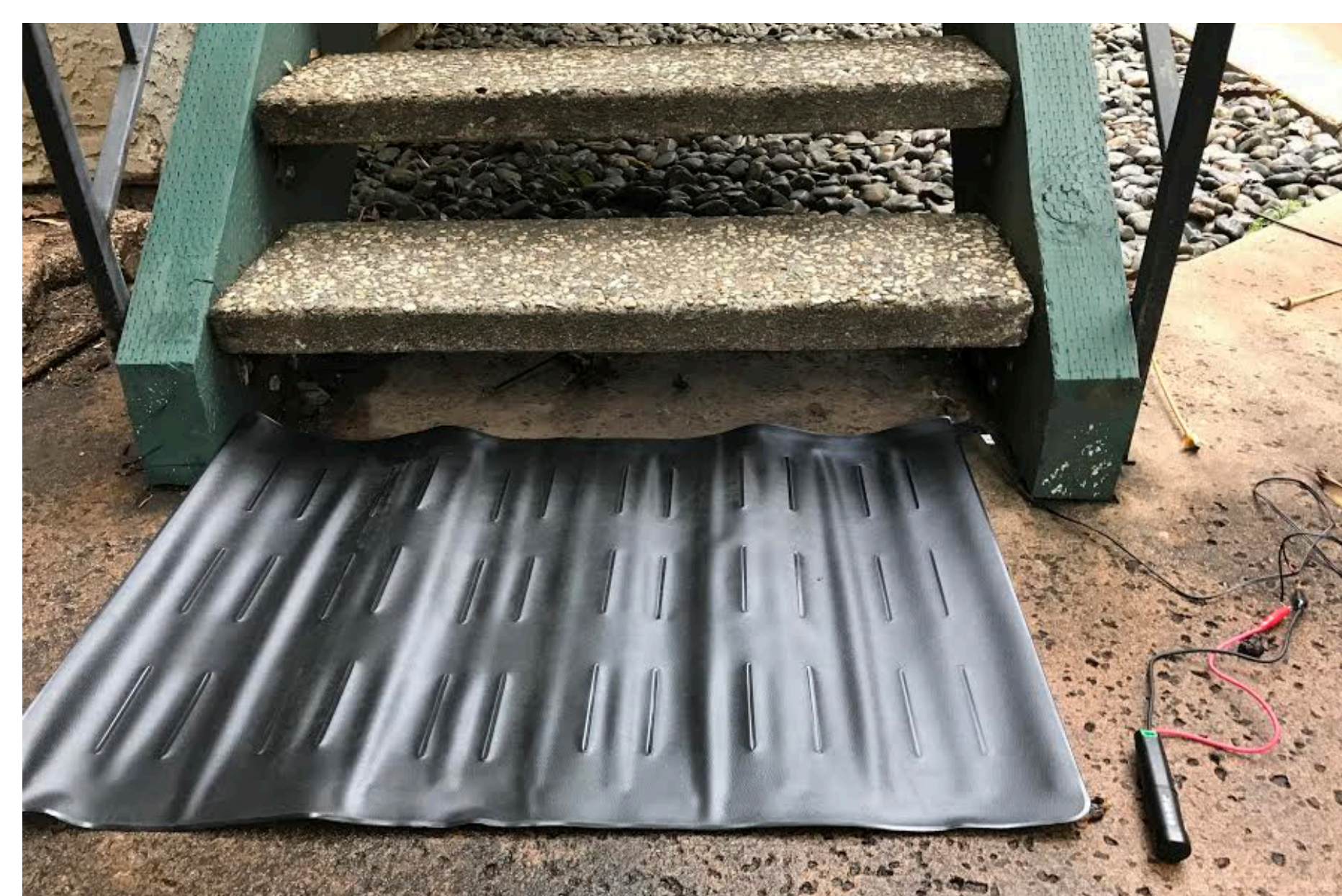
Figure 1. 24" x 36" wireless and wired mat with data logger.
