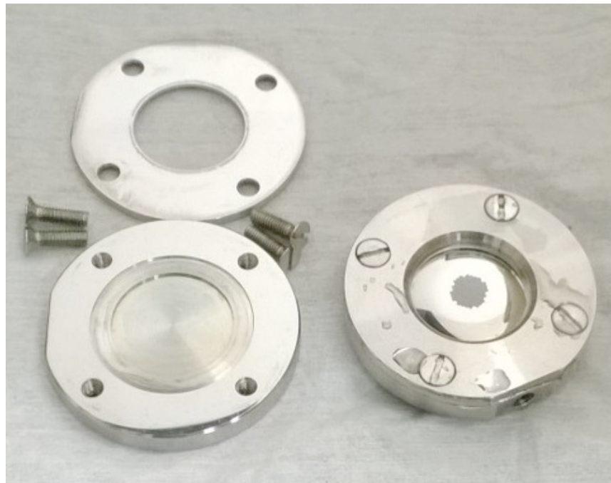
Figure 7.2 MCP jig supplied by Photonis before MCP insertion (left) and after removal from water rinse (right). Note the well can be observed in the left image, where backfilled water is placed. The mirror finish on the seal surrounding the MCP makes the jig water-tight.
