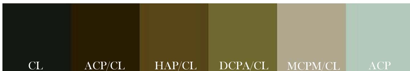
Fig. 2. Averaged color of pure CL, pure ACP and different CAP powders loaded with CL after their annealing to 200 °C in air, at the heating rate of 10 °C/min.
