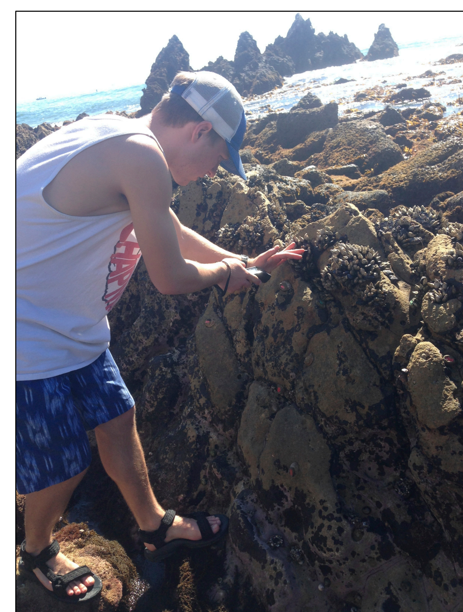
Figure 3. Measuring experimental and control limpet radiant temperatures with field-calibrated infrared "thermogun." Temperature measurements were taken every 15 minutes throughout the 3-hour heating period.
