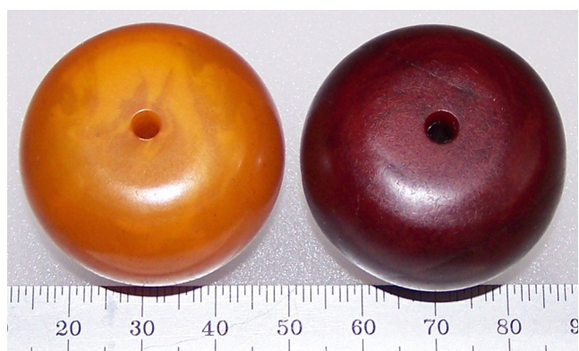
Figure 8. PF bead subjected to elevated temperatures in air (right) compared to an unheated one (left). Thermal cycle was 1 hour at 121 C, followed by 1 hour at 149 C, followed by 1 hour at 177 C.
