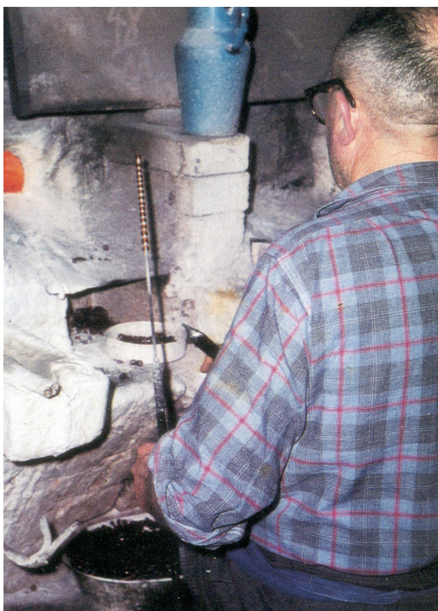
Figure 5. Beadmaker at the Lindner Trasslhütte in Warmensteinach, ca. 1960, with a series of beads on his mandrel (Herrmann 2008:28).
