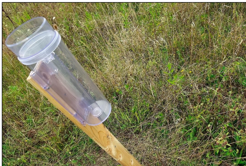
Figure 3-2: Rain gauge installed at the Skytop location
