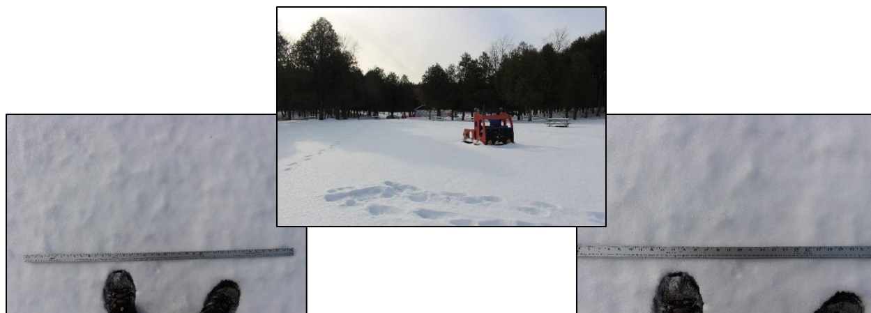
Figure 3-8: Standardized snow surface photos taken at the relocated second season E site: chest height (left), waist height (right) and site overview (center)
