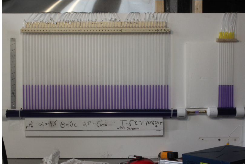
Figure A.3: The raw manometer panel images are scaled to include both the main panel and sub panel, the scale reference, and notes regarding the current model configuration and operating condition.
