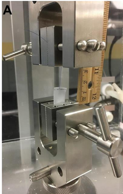
Figure 3-6 (A) Suture retention testing set-up and (B) representative force-displacement plot for the composite using a tensile speed of 50 \text{ mm} \cdot \text{min}^{-1} . The suture retention strength is denoted by an asterisk.
