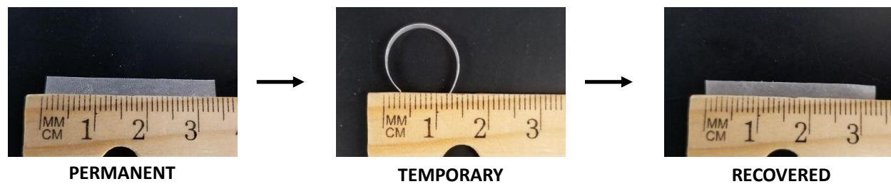
Figure 5-16. Qualitative demonstration of one way shape memory of the PVAc/PAH composite.
