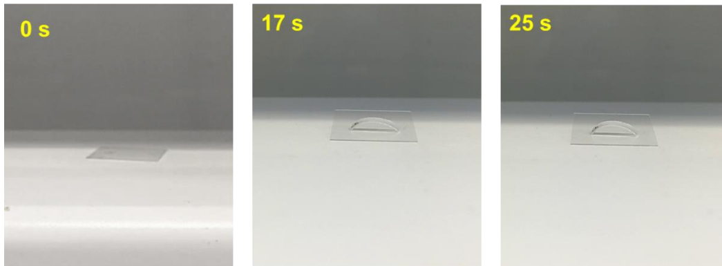
Figure 7-7. Time-lapsed mechanically programmed displacement of an object by the anisotropic PCL/epoxy composed of oriented PCL arranged orthogonally. A rectangular strip was topped with a glass cover slip and placed on a hot plate at 45 °C. As the mechanically programmed shape was thermally activated, the sample began to curl and lift the glass slide in under 30 s. The schematic above demonstrates the thermally activated sequence of free-standing object displacement by the sample shown below.
