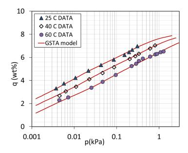
Figure 5-13. Fitting of GSTA model to the isotherms for AgZ.
