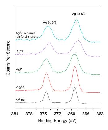
Figure 6-11. XPS spectra of Ag 3d for Ag standards and AgZ samples.
