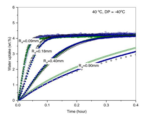
Figure 5-1. Uptake curves of  $H_2O$  adsorption on  $Ag^0Z$  of different particle radii at the temperature of 40 °C and dew point of -40 °C.
