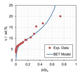
Figure 5-9. Comparison of BET model with the isotherm of  $H_2O$  adsorption on  $Ag^0Z$  obtained at 25 °C.
