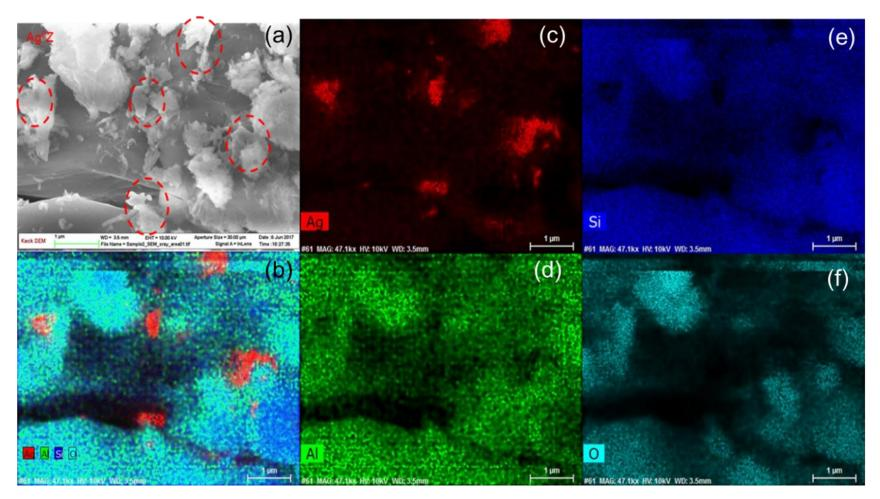
Figure 4-4. Element mapping of Ag<sup>0</sup>Z. a) Secondary electron imaging, b) overlapped mapping of Ag, Al, Si and O, c) mapping of Ag, d) mapping of Al, e) mapping of Si, f) mapping of O.
