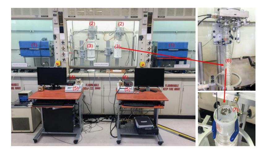
Figure 3-4. Photographs of the iodine adsorption systems. (1). Dynacalibrator; (2). Microbalance; (3). Furnace; (4). Temperature controller; (5). Data collection system; (6). Adsorption column with preheating coil inside the furnace; (7). Stainless steel screen tray with Ag<sup>0</sup>Z loaded.
