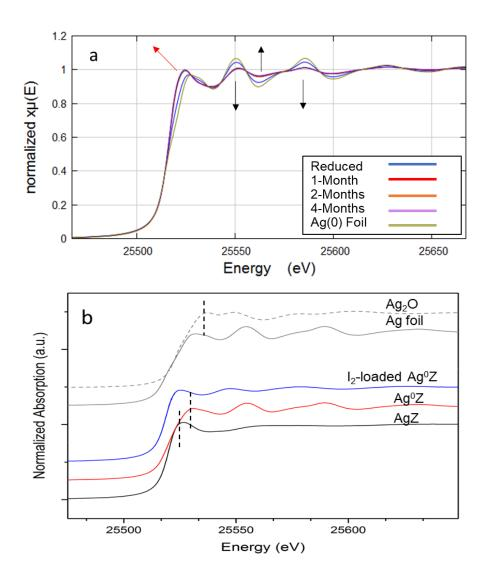
Figure 6-12. EXAFS of Ag<sup>0</sup>Z samples (a) and Ag standards (b).
