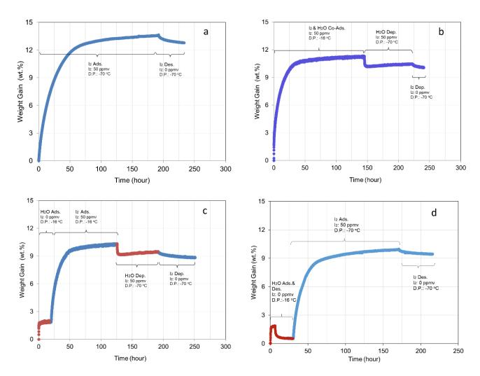
Figure 6-4. Adsorption and desorption of  $I_2$  and/or  $H_2O$  in different sequences. a)  $I_2$  adsorption followed by desorption. b)  $I_2/H_2O$  coadsorption followed by  $H_2O$  desorption and then  $I_2$  desorption. c)  $H_2O$  adsorption and then  $I_2$  adsorption followed by  $H_2O$  desorption and then  $I_2$  desorption. d)  $H_2O$  adsorption and then desorption followed by  $I_2$  adsorption and then desorption.
