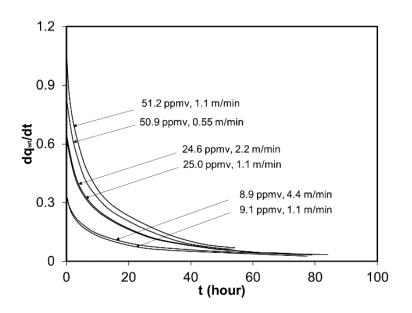
Figure 4-10. Comparison of the uptake rates of uptake curves in Figure 4-9.  $q_{wt}$  (wt. %) is the concentration of I<sub>2</sub> in Ag<sup>0</sup>Z.
