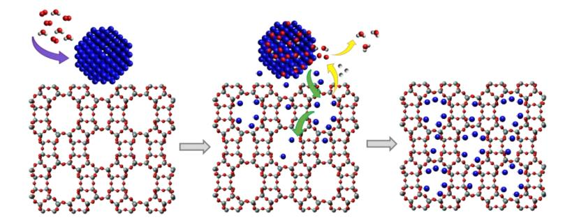
Figure 6-13. Deactivation pathway of  $Ag^0Z$  in humid air.
