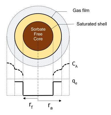
Figure 3-7. Shrinking core process during adsorption on a solid particle.
