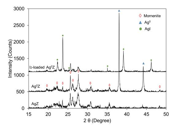
Figure 4-7.XRD patterns of AgZ,  $Ag^0Z$  and  $I_2$ -loaded  $Ag^0Z$ .
