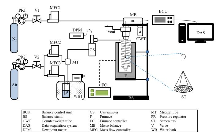
Figure 3-5. Schematic diagram of the continuous flow water adsorption system.
