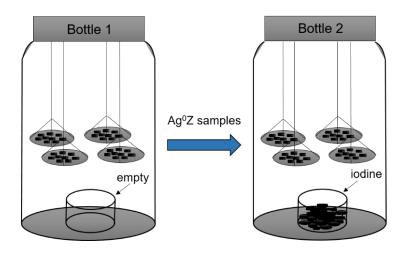
**Figure 3-2**. Batch experimental setup for comparing the capacities of  $Ag^0Z$  reduced at different conditions. After  $Ag^0Z$  were pre-equilibrated in Bottle 1, they were transferred to Bottle 2 for I<sub>2</sub> adsorption.
