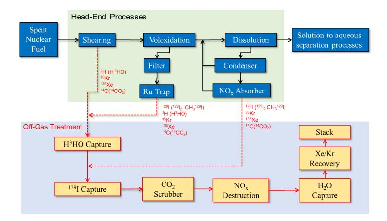
Figure 1-1. Head-end processes of spent nuclear fuel reprocessing and off-gas treatment systems.<sup>7</sup>
