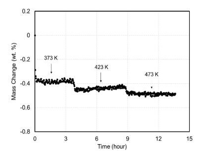
Figure 4-13. Desorption of H<sub>2</sub>O when Ag0Z is equilibrated in dry air stream (dew point: -  $70^{\circ}$ C) at 100 (373 K), 150 (423 K), and 200 °C (473 K), sequentially.
