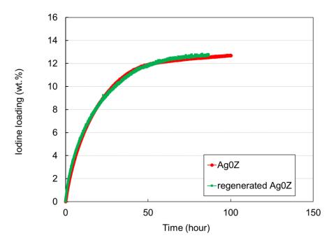
Figure 4-16. I<sub>2</sub> adsorption on  $Ag^0Z$  and regenerated  $Ag^0Z$
