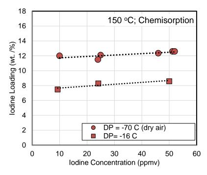
Figure 6-2. Isotherms chemisorption of  $I_2$  on AgZ in the dry and humid air.
