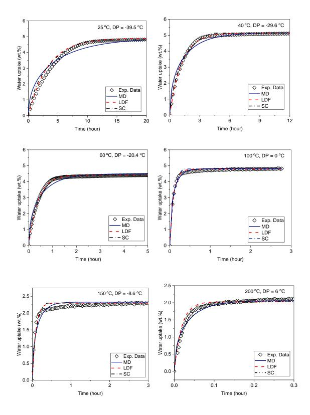
Figure 5-7. Curve-fitting of the MD, LDF and SC models to the uptake curves of  $H_2O$  on  $Ag^0Z$  at different conditions.
