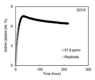
Figure 4-14. Uptake curves of  $I_2$  adsorption on  $Ag^0Z$  at 250 °C (523K). A decrease in mass is observed from 35 hours without stopping  $I_2$  in the gas stream which is due to possible decomposition of AgI.
