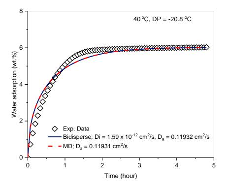
Figure 5-5. Comparison of the bidisperse and macropore diffusion models to fit the uptake curve of  $H_2O$  on  $Ag^0Z$  pellets (0.9 mm) at 40°C over the dew point of -20.8 °C. The prediction curves of the two models overlapped in the plot.
