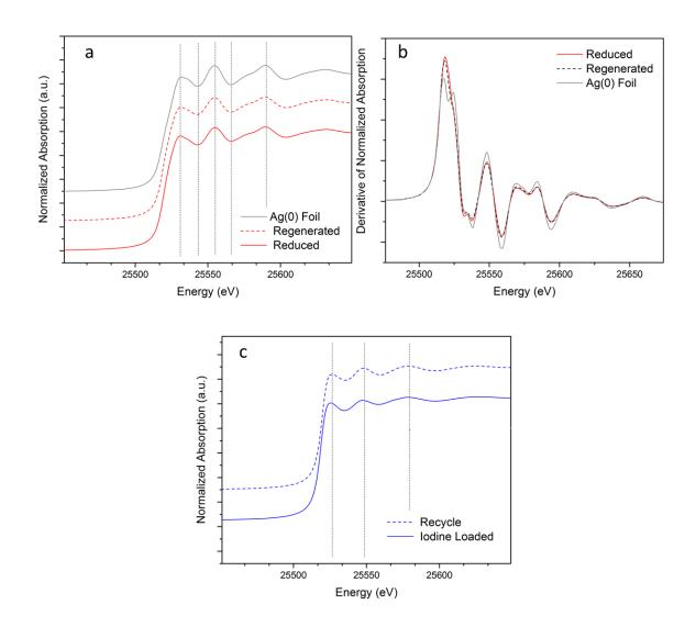
Figure 4-17. XANES spectra for  $Ag^0Z$  samples. a) Normalized spectra of  $Ag^0Z$ , regenerated  $Ag^0Z$  and Ag foil samples. Dashed grey lines are drawn at characteristic spectral features. b) The derivative of the XANES spectra in a). c) Normalized spectra of I<sub>2</sub>-loaded  $Ag^0Z$  and I<sub>2</sub>-loaded regenerated  $Ag^0Z$  (Recycle).
