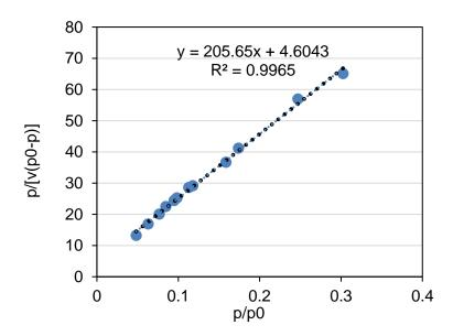
Figure 5-10. The plot of  $p/[v(p_0-p)]$  vs.  $p/p_0$  using the H<sub>2</sub>O adsorption data on Ag<sup>0</sup>Z obtained at 25°C and relative pressures between 0.05-0.3.
