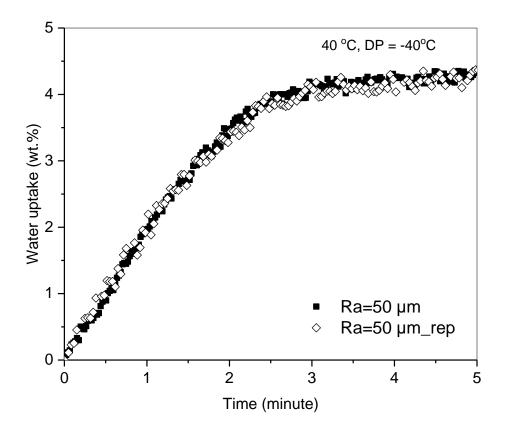
Figure 5-3. Adsorption of H<sub>2</sub>O vapor on Ag<sup>0</sup>Z powder ( $R_a = 50 \mu m$ ) at the temperature of 40 °C and dew point of -40 °C.
