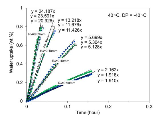
Figure 5-2. The initial fractional uptake rate of  $H_2O$  vapor on  $Ag^0Z$  was inversely proportional to the radius of the  $Ag^0Z$  particles, which indicated that the adsorption process was controlled by macropore diffusion.
