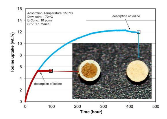
Figure 4-8. A comparison of the cross-section of  $Ag^0Z$  fully loaded with  $I_2$  and that partly loaded with  $I_2$ . The clear interface observed in the  $Ag^0Z$  partly loaded with  $I_2$  suggests that the adsorption process is a shrinking core process.
