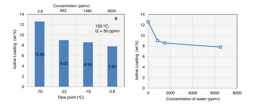
Figure 6-3.  $I_2$  adsorption capacity (chemisorption) of  $Ag^0Z$  in humid air streams of different dew points.  $I_2$  was co-adsorbed with  $H_2O$ .
