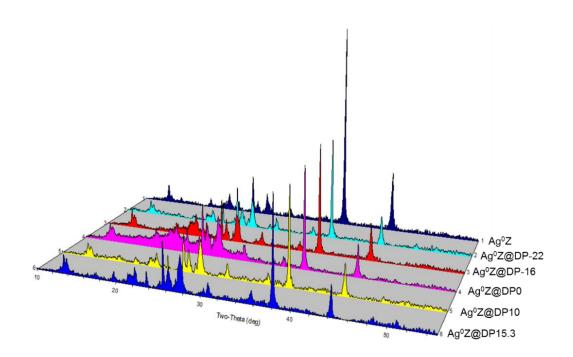
Figure 6-5. XRD patterns of Ag<sup>0</sup>Z and Ag<sup>0</sup>Z treated in humid air flows of different dew points for 24 hr at 150 °C
