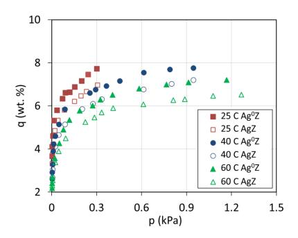
Figure 5-12. Isotherms of H<sub>2</sub>O adsorption on AgZ and Ag<sup>0</sup>Z.
