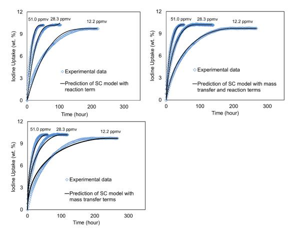
Figure 4-15. Comparison of the prediction of the SC model with different combinations of rate controlling terms.
