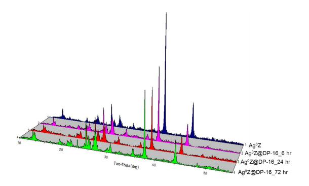
Figure 6-6. XRD patterns of  $Ag^0Z$  and  $Ag^0Z$  treated in the humid air flow of dew points - 16 °C for different periods at 150 °C.
