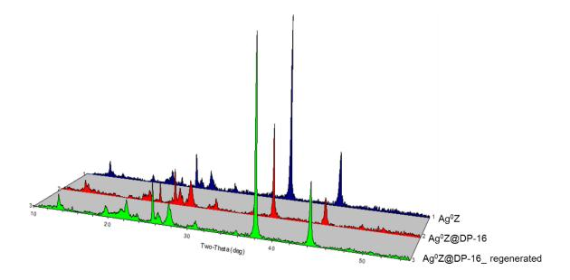
Figure 6-7. XRD patterns of  $Ag^0Z$ ,  $Ag^0Z$  treated in the humid air flow of dew points -16 °C for 24 hr at 150 °C and consequently regenerated  $Ag^0Z$ .
