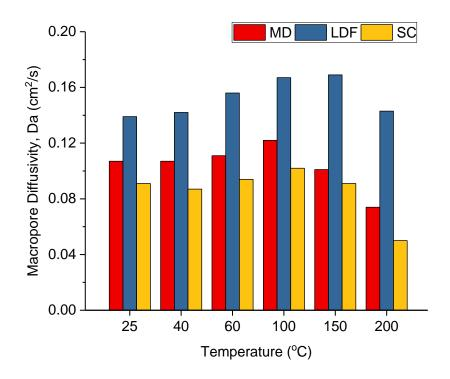
Figure 5-8. Comparison of the macropore diffusivity obtained using the MD, LDF and SC models.
