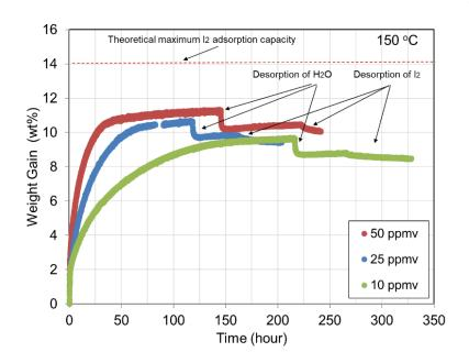
Figure 6-1. Co-adsorption of  $I_2$  and  $H_2O$  on  $Ag^0Z$  followed by desorption of  $H_2O$  and  $I_2$ .
