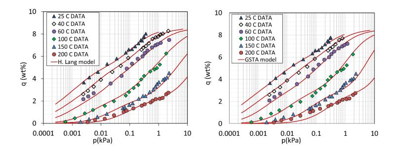
Figure 5-11. Isotherms of H<sub>2</sub>O adsorption on Ag<sup>0</sup>Z obtained at 25, 40, 60, 100, 150, and 200 °C and fitted by the Heterogeneous Langmuir (left) and GSTA (right) models.
