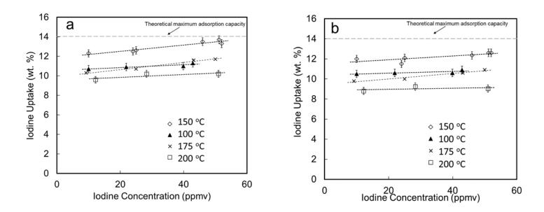
Figure 4-12. Isotherms of  $I_2$  adsorption on  $Ag^0Z$ . a) Total adsorption; b) Chemisorption.
