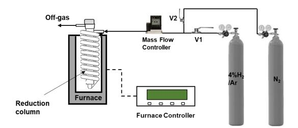
Figure 3-1. Experimental setup for reduction of AgZ.
