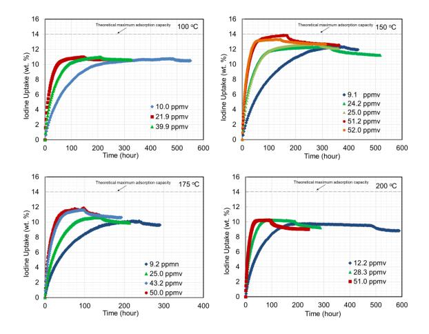
Figure 4-11. Uptake curves of  $I_2$  adsorption on Ag0Z at 100, 150, 175, and 200 °C, over  $I_2$  concentration between 9 - 52 ppmv.
