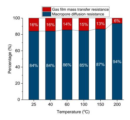
Figure 5-6. Distribution of mass transfer resistances for  $H_2O$  adsorption on 0.9 mm Ag<sup>0</sup>Z pellets.
