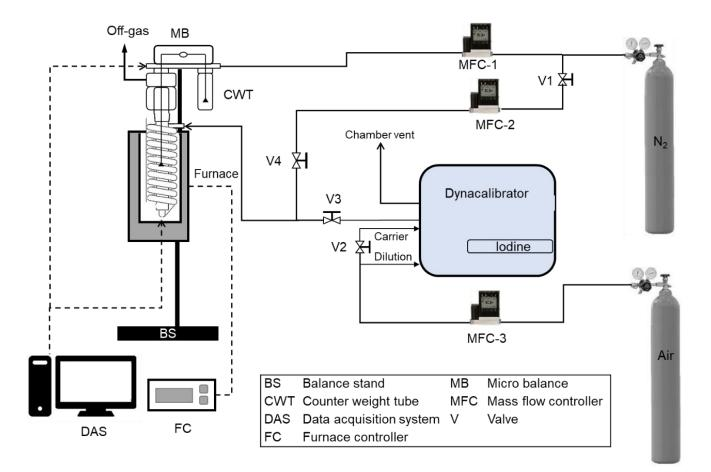
Figure 3-3. Schematic diagram of the continuous-flow I<sub>2</sub> adsorption system.
