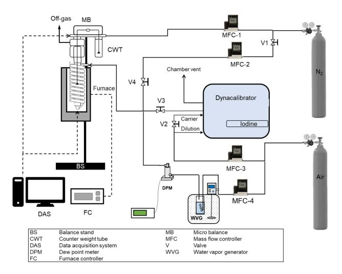
**Figure 3-6.** The modified adsorption system for I<sub>2</sub> - H<sub>2</sub>O co-adsorption.
