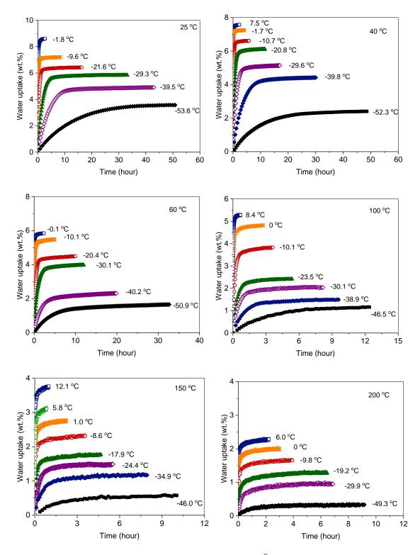
**Figure 5-4**. Uptake curves of  $H_2O$  vapor on 0.9 mm  $Ag^0Z$  in gas streams at temperatures from 25 to 200 °C and dew points from -53.6 - 12.1 °C.
