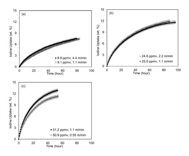
Figure 4-9. Effect of gas velocity on the uptake rate of  $I_2$  on  $Ag^0Z$  at 150 °C with different  $I_2$  concentrations in the gas stream.
