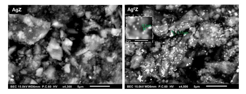
Figure 4-3. SEM (backscattered election composition) images of AgZ and  $Ag^0Z$
