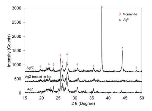
Figure 4-5. XRD patterns of AgZ and  $Ag^0Z$
