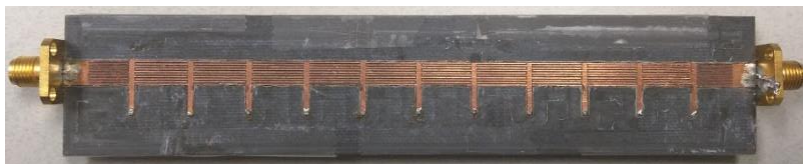
Figure 4-5 A 10-unit-cell CRLH TL transitioned to a 50 Ohm microstrip line without tapering.
