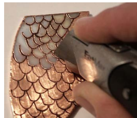
Figure 3: Cut away surplus copper foil with a craft knife or razor blade.
