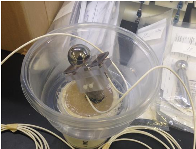
Fig. 97: 1 st generation potting system and environmental chamber with sensors and target fixed to the implant.
