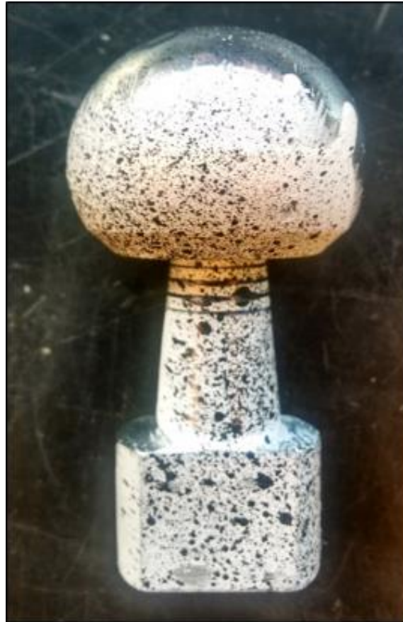
Fig. 18: Test sample spray painted with speckle paint. Specks were used during displacement analysis.
