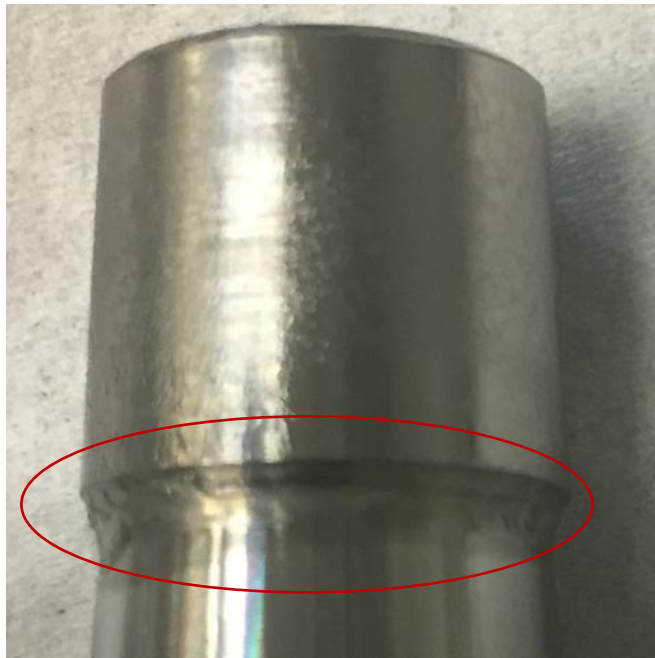
Fig. 80: Coagulated ring buildup of liquid lipids about the base of the trunnion post testing. The image indicates a significant amount of the applied contaminant is squeezed out of the taper junction during seating.
