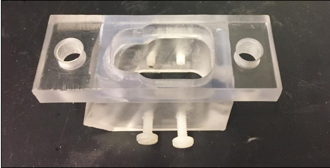
Fig. 96: 1 st generation sensor fixture. Holds two eddy current sensors fixed to the stem targeting the head.
