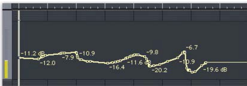
Figure 30. Illustration of volume automation. From (Bennett, 2005).
