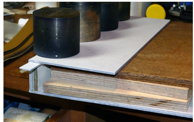
Attaching the lids with spacer inserted and lid supported to facilitate weighing down.
