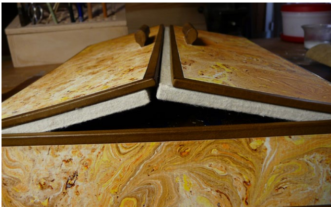
Padding attached to the lids with offset to prevent dust from entering.
