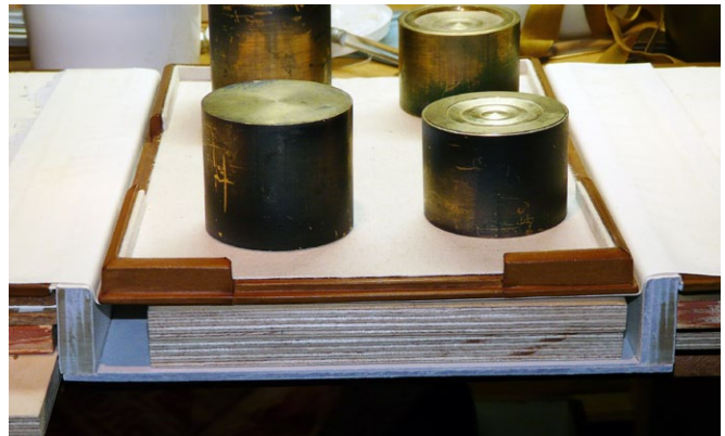
The lids must be horizontal while attaching the base. Boards under the base are used to hold it in place and level while the "lift" fabric is being secured to the lids.
