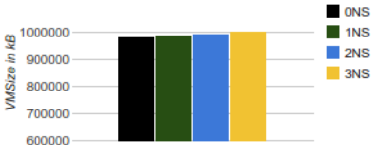
Figure 5.14: Average memory footprint in kB (VmSize) for 0-, 1-, 2- and 3-namespace configurations.
