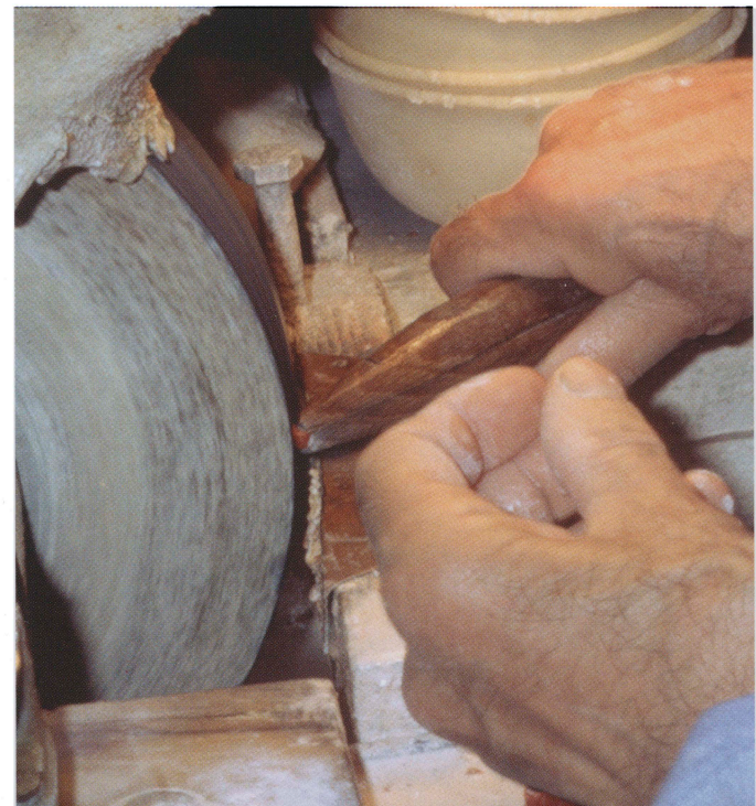
Plate ID. Coral: Shaping beads using an electric carborundum grinding wheel with the coral piece held tight in a wooden pliers ( pliorsor ) or attached to a stick with resin. This rounds the rough edges and removes the rest of the soft crust. The final form is achieved in subsequent grinding stages (photo by author).
