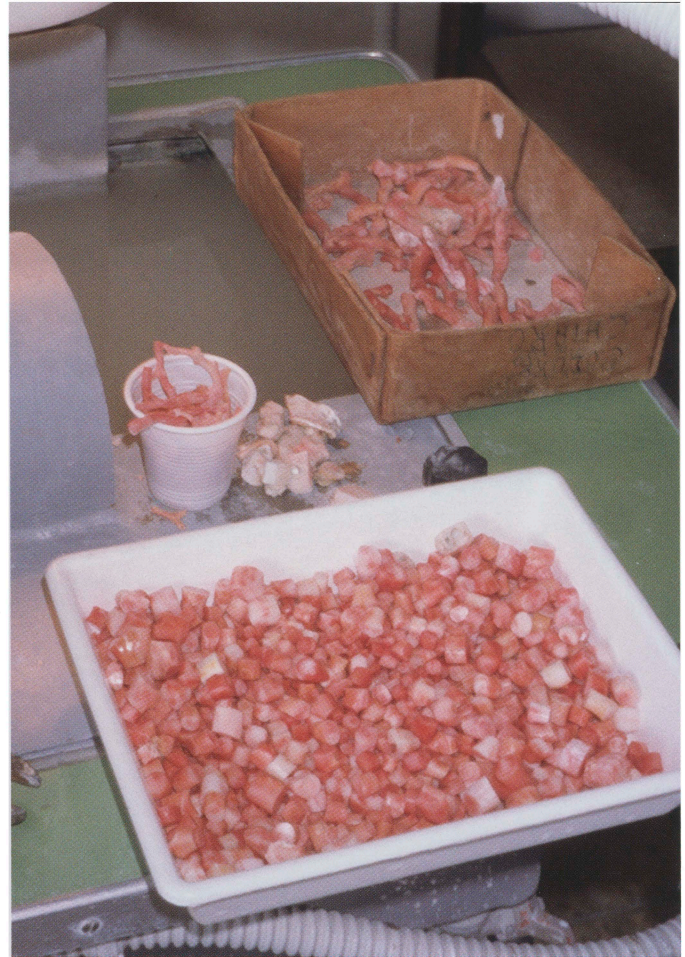
Plate IB. Coral: Cerasuolo coral branch fragments (rear) and the blanks cut from them (front). Three stages of production can be seen here. The coral branches have been cut into bead blanks and sorted into more refined groups by color and shape. These first steps of examination, and branch and blank cutting, are considered the most important in the entire production process (photo by author).
