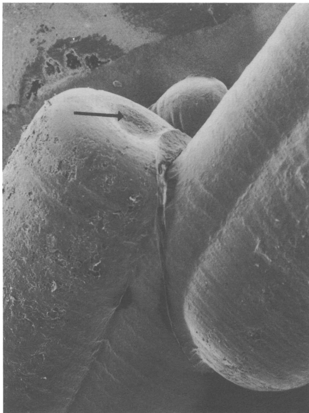
Figure 9. The leading edge of a drill hole which was probably made with a rod. The central depression (arrow) represents a slight elevation in the stone caused by a depression in the end of the drill. Shallow concentric grooves in the side wall can be attributed to abrasive which would have been used with a rod-shaped drill.
