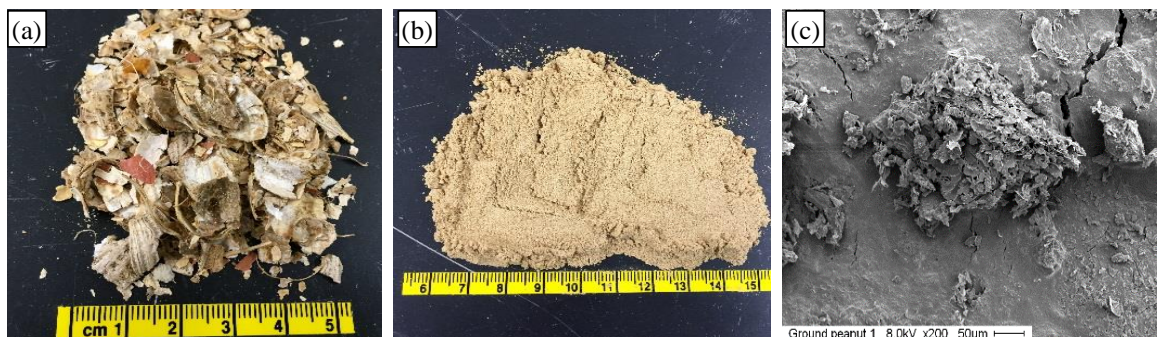
Figure 2.1 (a) Peanut husk, (b) Ground peanut husk, and (c) SEM image of ground peanut hull
