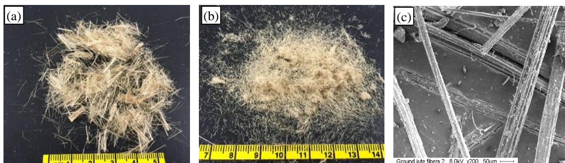
Figure 2.2 (a) Jute fibers, (b) Ground jute fibers, and (c) SEM image of ground jute fibers
