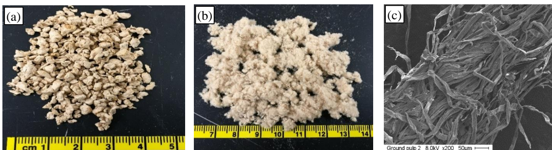
Figure 2.3 (a) Kraft pulp, (b) Ground kraft pulp, and (c) SEM image of ground kraft pulp
