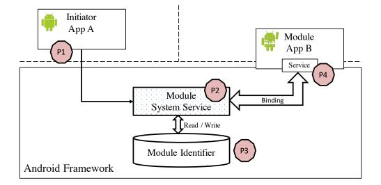
Fig. 4.1.: Design Architecture of Framework Module on Android
