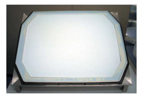
Fig. 1.2. NaI scintillation crystal. [5]
