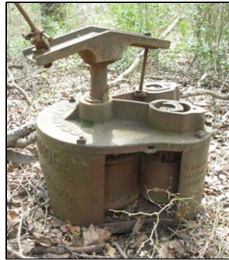
Figure 5.18: Ribbon cane syrup mill and Chattanooga No. 8 cane press located north of the Taylor Household (S. Loftus).
