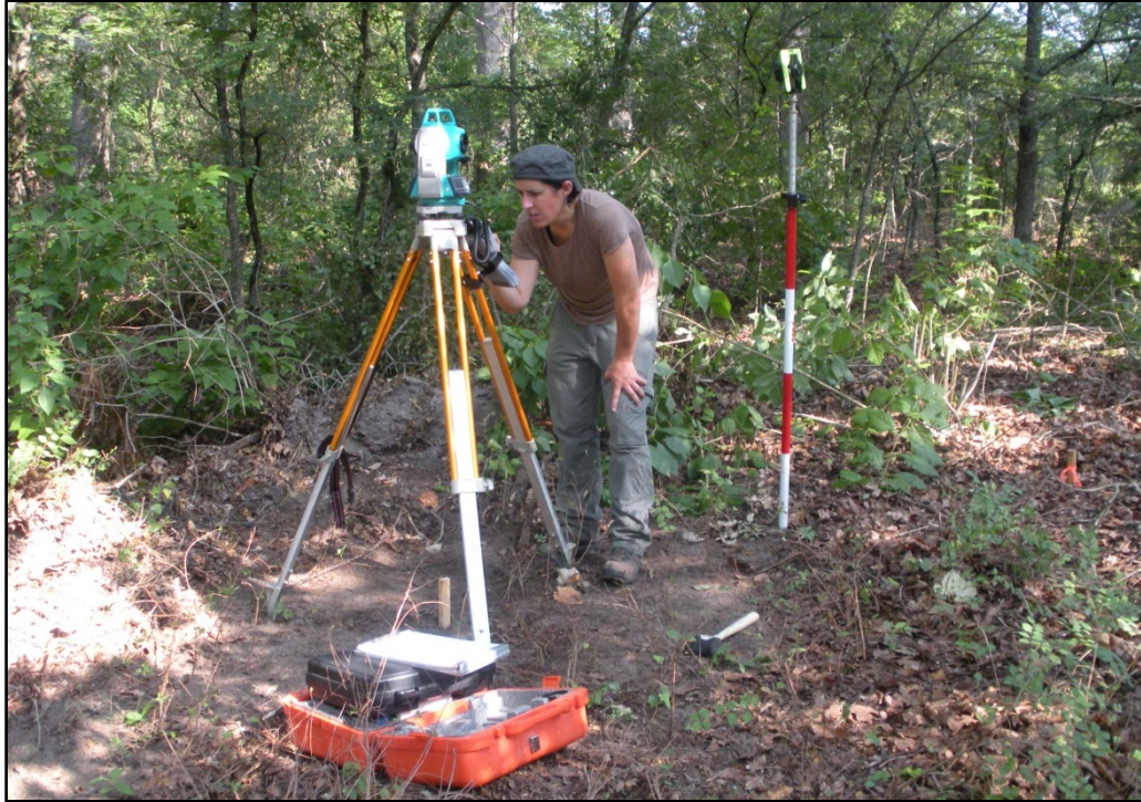
Figure 4.4: Sarah Loftus using the Total Station to establish a grid at the Davis Household (J. Shipp).
