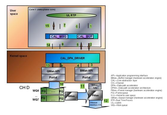
Figure 20: Egress Data Plane IP Packet Processing
