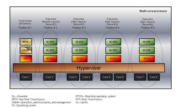
Figure 8: Supervised Asymmetric Multi-Processing (S-AMP) Configuration
