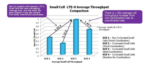
Figure 7: LTE-U Small Cell Average Throughput Comparison
