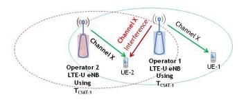
Figure 3: Multi-Operator LTE-U Co-channel Interference Scenario
