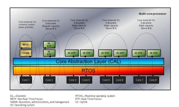
Figure 10: Deterministic Symmetric Multi-Processing (D-SMP) Configuration
