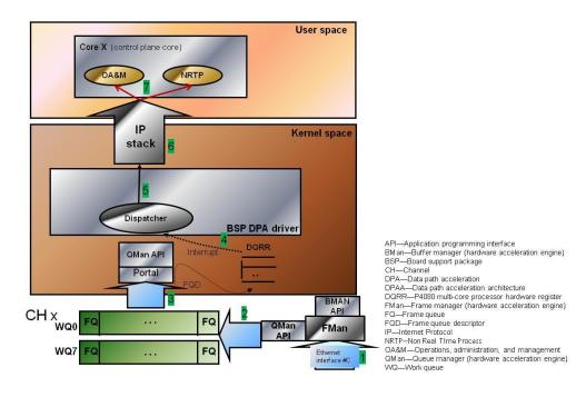
Figure 17: Ingress Control Plane IP Packet processing using Protocol Stack
