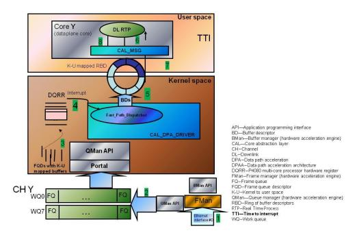
Figure 19: Ingress Data Plane IP Packet Processing
