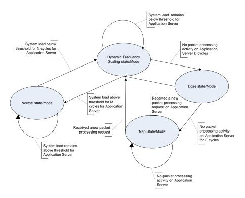
Figure 12: DPC State machine for the dedicated data plane cores
