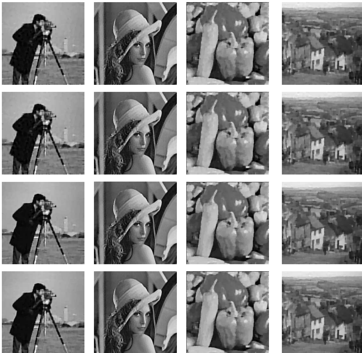
Figure 4.18: Recovered images of “Cameraman”, “Lena”, “Peppers”, and “Goldhill” (from top row to bottom row) with the \ell_1 -TV model for images blurred by the (15, 10)-GBM and corrupted by impulsive noise of level p = 0.5 . Row 1: the CP; Row 2: the ZBO; Row 3: Algorithm 2; Row 4: Algorithm 1.
