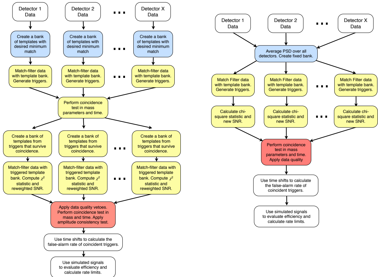
Figure 35: These flowcharts describe the topologies for the pipeline used in the S6 search (left) and the final configuration described here (right). Each color represents a distinct modification made to the pipeline described in the different sections in the chapter. The yellow is described in Sec. 7.4.1, the blue in Sec. 7.4.3 and the red in Sec. 7.4.4.
