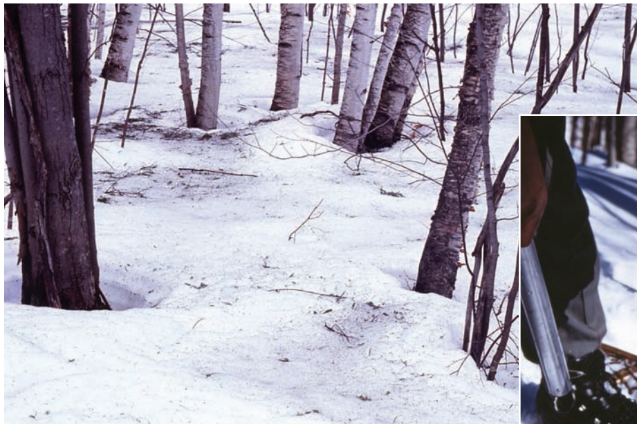
Snow cores are collected and weighed to measure the water content of snow. Photographs: U.S. Forest Service Archives
