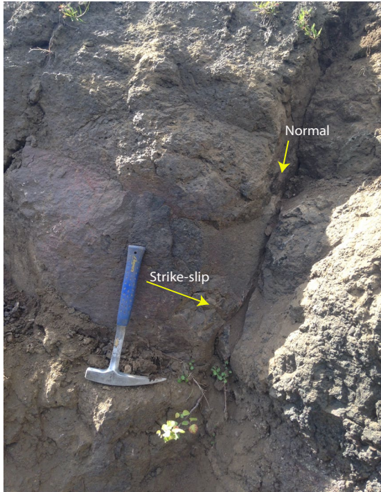
Figure 15. Strike-slip features seen in the field. A) Normal fault plane cutting a strike-slip fault plane. B) Micromylonitic (glassy) features seen in the lower right above the pencil. These preserve horizontal slickensides in this picture. C) Right-lateral fault plane. Black dashed lines parallel slickenlines and yellow dotted lines indicate Riedel shears.
