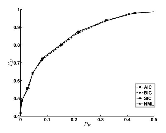
Fig. 5.2: ROC comparing the different MDL-based selection criteria.
