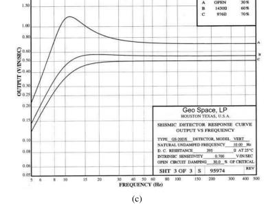
Fig. 2.1: The GS 20DX geophone. (a) Sensor as housed and packaged (b) Electrical details: cable length and sensor polarity (c) Frequency response curve.
