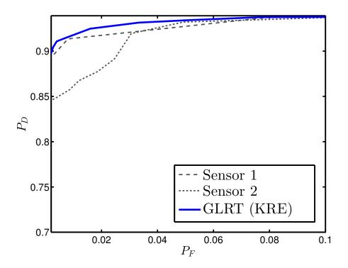
Fig. 4.7: ROC for Background vs. Footstep detection.
