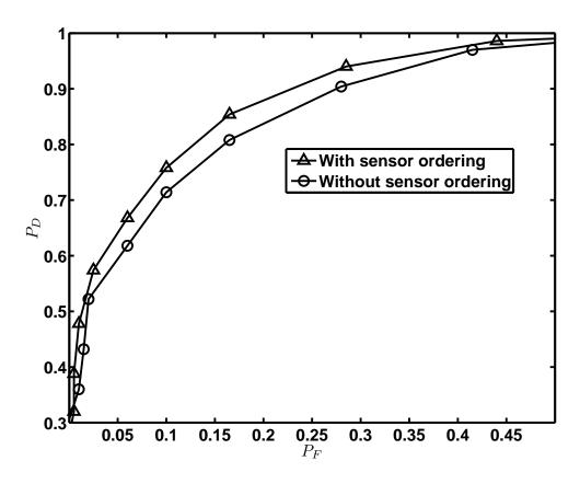
Fig. 5.4: ROC illustrating the benefit of using  $\lambda_U$ -based node ordering.
