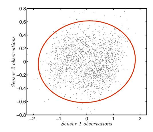
Fig. 4.5: Scatter plot of pilot background data (5000 observation pairs). The 99% confidence ellipse is shown for a  $\mathcal{N}([0,0]^{\mathsf{T}},\Sigma)$  distribution, where  $\Sigma_{1,1} = 0.58$ ,  $\Sigma_{1,2} = \Sigma_{2,1} = 0.009$  and  $\Sigma_{2,2} = 0.05$  are the elements of the covariance matrix  $\Sigma$ .
