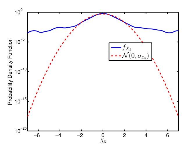
Fig. 2.7: Probability distribution of the footstep data from Sensor 5, compared to the p.d.f. of normal distribution with the same second-order moments as the footstep data. The Y-axis is plotted on a logarithmic scale.
