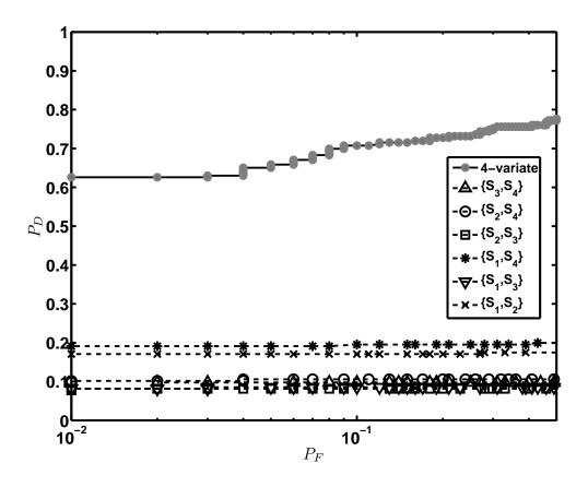
Fig. 5.5: ROC comparing multivariate copula based detector to various bivariate copula based detectors.  $\{S_p, S_q\}$  represent sensor pairs for p, q = 1, 2, 3, 4 and  $p \neq q$ . The x-axis is on a logarithmic scale to emphasize low  $P_F$  values.
