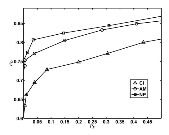
Fig. 5.3: ROC comparing the different detectors obtained from different marginal models. SIC is used for copula selection. CI: Complete Ignorance, AM: Approximate Modeling, NP: Nonparametric modeling.
