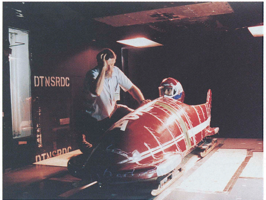
As a member of the U.S. Bobsled Federation, Professor Jerome Malinowski assists the Olympic bobsled team with innovative sled design. Here he tests the aerodynamics of a new sled in the wind tunnel of David Taylor Research Center in Maryland.
