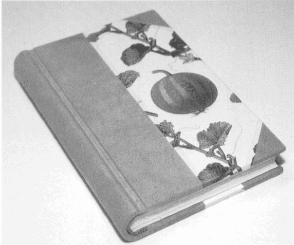
Fig. 17. Completed full cloth binding
