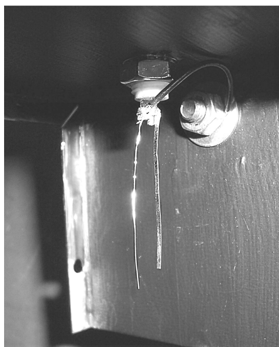
Figure 2. 5: Electrodes. Wire (ground) / Strip (measuring) configuration shown.
