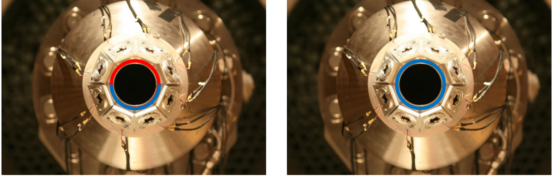
Figure 3.18: Fourier-azimuthal forcing mode 1 (left) and mode 0 (right)
