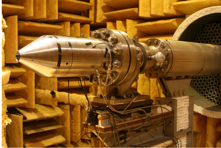
Figure 2.2: High-speed jet rig within Syracuse University anechoic chamber
