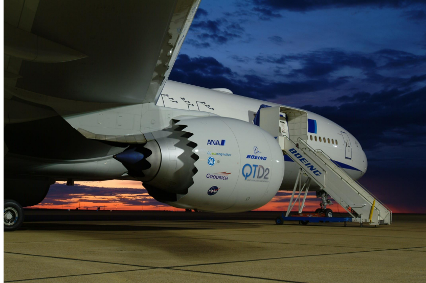
Figure 3.2: NASA chevron design on GE engine for noise reduction, Banke (2009) [22]
