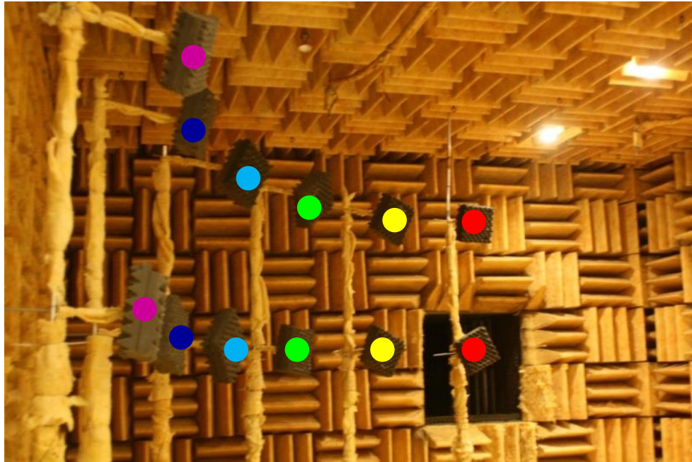
Figure 5.57: Far-field microphone configuration
