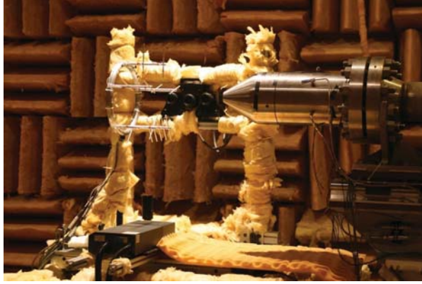
Fig. 3 Large Window PIV Setup
