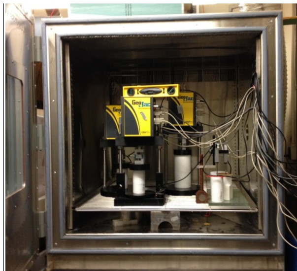
Figure 99. Set up of creep test inside chamber
