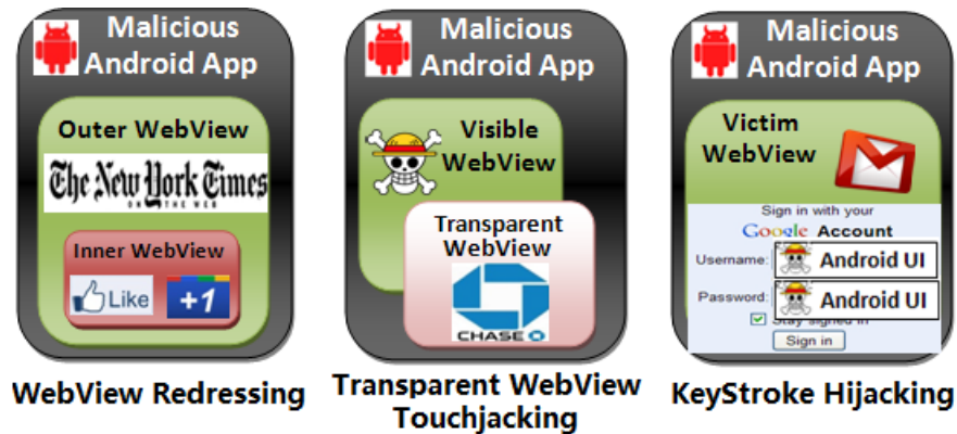
Fig. 5.4.: Touchjacking Attack Overview
