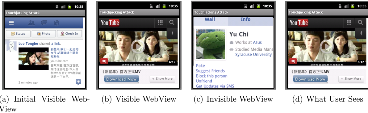
Fig. 5.7.: Invisible WebView Attack Example
