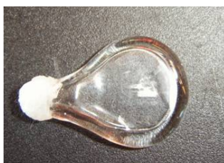
Figure 1: A fabricated tear-shaped glass holder in lab. The narrow neck allows the temperature probe to be inserted and prevention of sample from leaking out. It is wide enough to allow the insertion of the sample into the deeper part of the glass holder.
