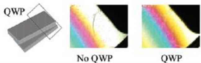
Figure 9: A wedge-shaped cell when placed under a polarizable microscope, expects to see certain results when there is no QWP and change in interference color when inserted QWP.
