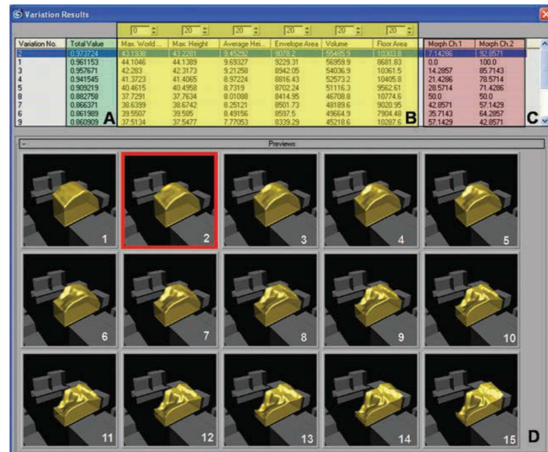
Figure 3: User interface, initial set up and generated alternatives visual interactive catalogue (the alternative with the highest grade in the current fitness settings is marked by a dark/red rectangle).
