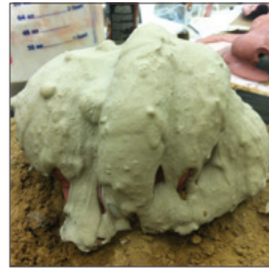
A MIX OF CEMENT, SAND, AND DYE IS POURED OVER TOP
