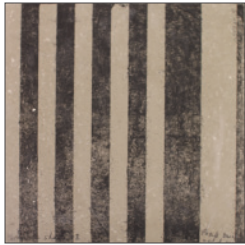
I ADDED GRAPHITE TO A CONCRETE MOLD AND IT IMPRINTED ON THE CONCRETE WHEN IT SET
