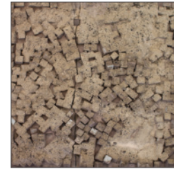
I USED FOAM BLOCKS AS AN AGGREGATE TO YIELD A CONCRETE PANEL 30% LIGHTER THAN TYPICAL CONCRETE
