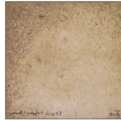
I USED SAWDUST AS AN AGGREGATE TO YIELD A CONCRETE PANEL 20% LIGHTER THAN TYPICAL CONCRETE
