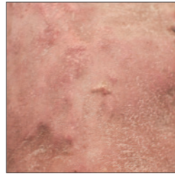
I USED FABRIC DYE TO COLOR THE SAND IN CONCRETE TO MAKE IT PINK
