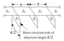
Figure 3.2: The structure of the shorted stub BPF
