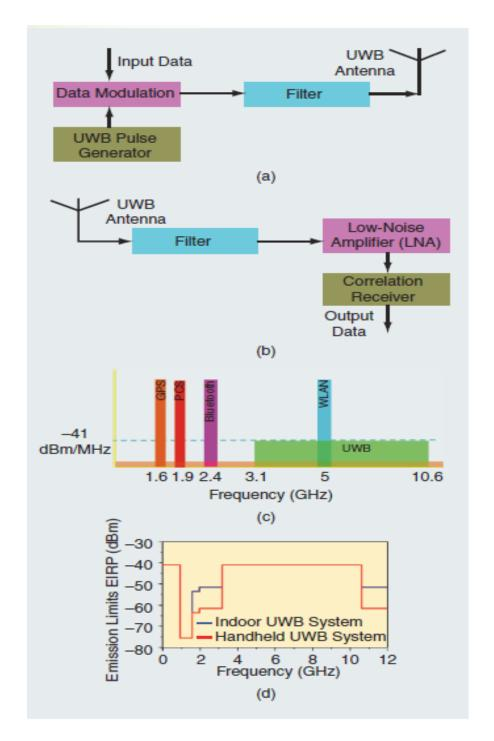
Figure 2.1: UWB system: (a) Transmitter, (b) Receiver, (c) Licensed and unlicensed band around the UWB spectrum, (d) FCC mask
