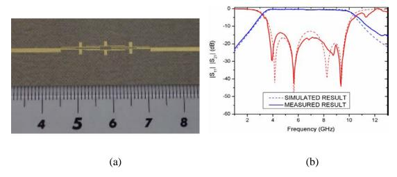
Figure 2.5: Filter using Microstrip Stub-Loaded Dual-Mode Resonator Doublets:
