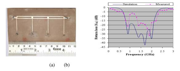
Figure 2.6: Filter using short circuited stubs: (a) Prototype, (b) Filter Performance
