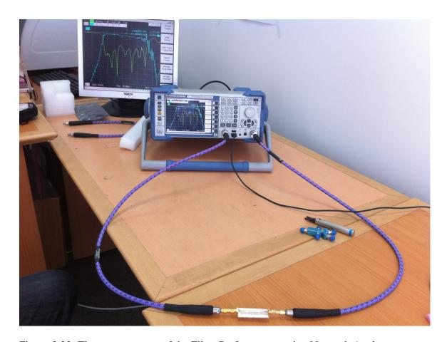
Figure 3.22: The measurement of the Filter Performance, using Network Analyzer
