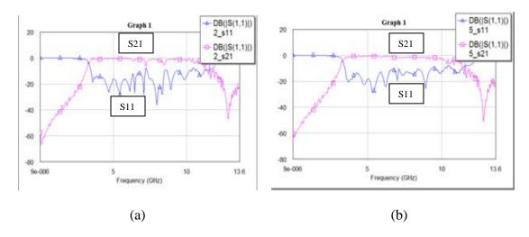
Figure 3.23: Measured S-Parameters of the Filter (a-before tuning, b-after tuning)
