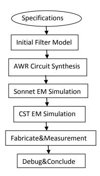
Figure 3.1: Flowchart of the design procedure
