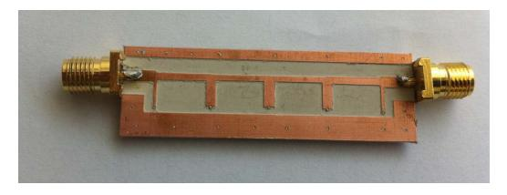
Figure 3.21: Fabricated Filter
