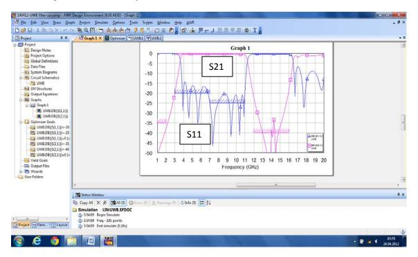
Figure 3.6: Optimized AWR Simulation Result
