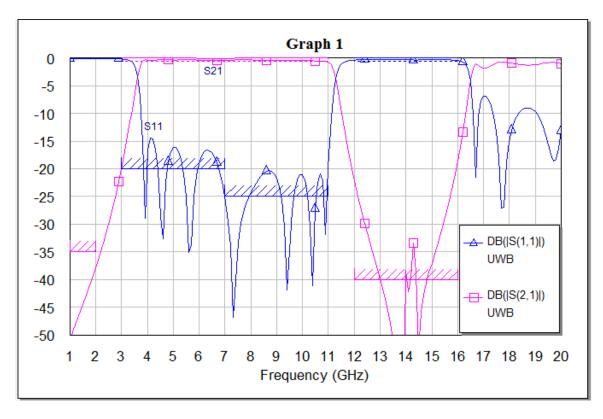
Figure 3.16: Final AWR Simulation Result
