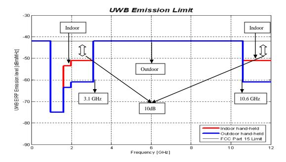
Figure 1.1: FCC Frequency Mask for UWB Applications
