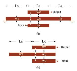
Figure 2.12: Multiline coupled line filter sample
