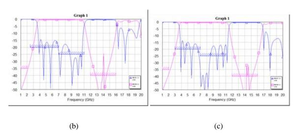
Figure 3.18: AWR Simulation Results for linewidth variations, (a) Nominal case, (b) linewidths +10%, (c) linewidths -10%.
