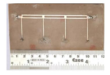
Figure 2.14: Sample filter with Shorted Stubs
