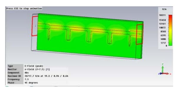
Figure 3.12: E- Field View of the filter, using CST EM Simulation
