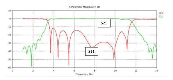
Figure 3.10: CST EM Simulation Analysis Result
