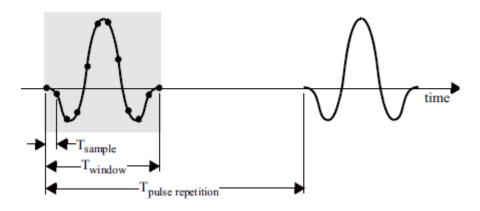
Figure 1.2: Representation of UWB pulses
