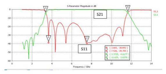
Figure 3.19: CST EM Simulation Results after decreasing the linewidths by %5
