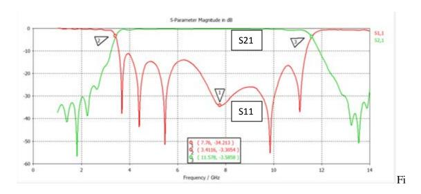
gure 3.20: CST EM Simulation Results after increasing the linewidths by %5
