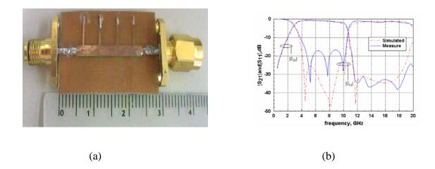
Figure 2.4: Filter using Hybrid Microstrip DGS: (a) Prototype, (b) Filter Performance
