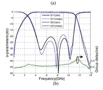
Figure 2.7: Filter using Parallel-Coupled Microstrip Lines: (a) Prototype, (b) Filter Performance
