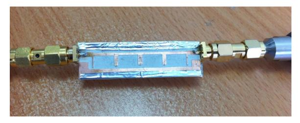
Figure 3.25: The final view of the filter at the final measurement process
