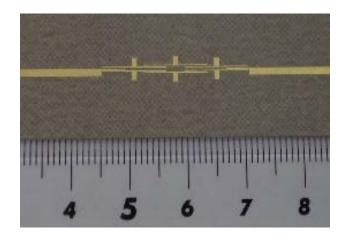
Figure 2.15: Sample filter with Resonator Doublets
