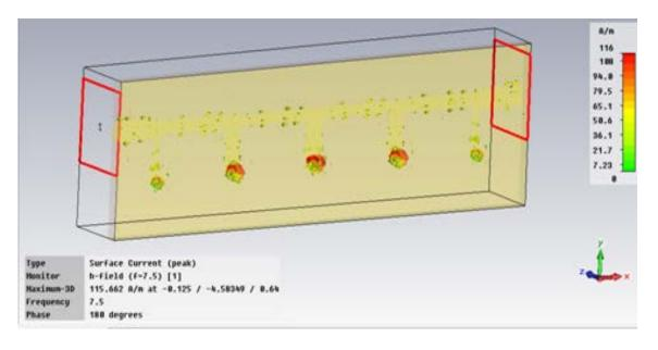
Figure 3.13: Surface Current View of the filter, using CST EM Simulation
