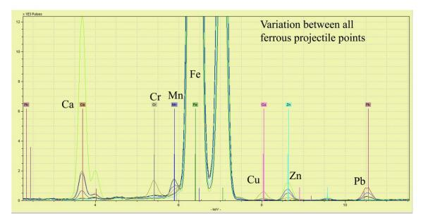
Figure 5:24 Variation visible in raw data pXRF spectroscopy of ferrous projectile points recovered from Fort Michilimackinac.
