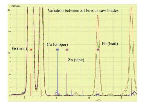
Figure 5:26 Variation visible in raw data pXRF spectroscopy of ferrous saw blades recovered from Fort Michilimackinac.
