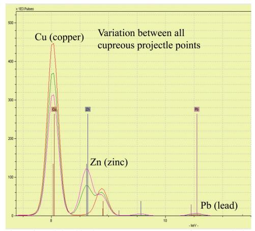
Figure 5:25 Variation visible in raw data pXRF spectroscopy of cupreous projectile point recovered from Fort Michilimackinac.
