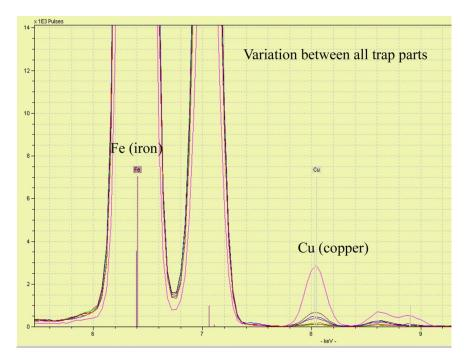
Figure 5:27 Variation visible in raw data pXRF spectroscopy of trap parts recovered from Fort Michilimackinac.
