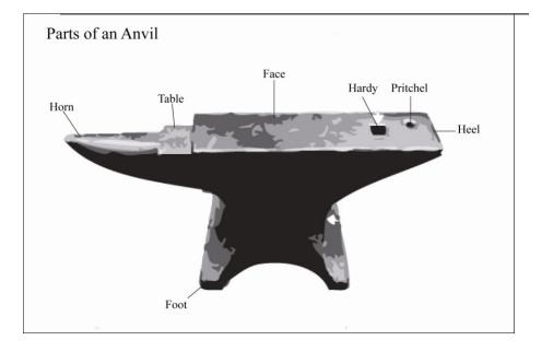
Figure 3:4 Parts of an anvil. Redrawn from Watson 2000, Andrews 1977 and Hawley 1976.
