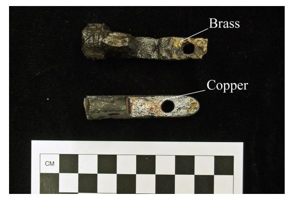
Figure 5:2: Breech plugs brazed with brass and copper (photograph by author).
