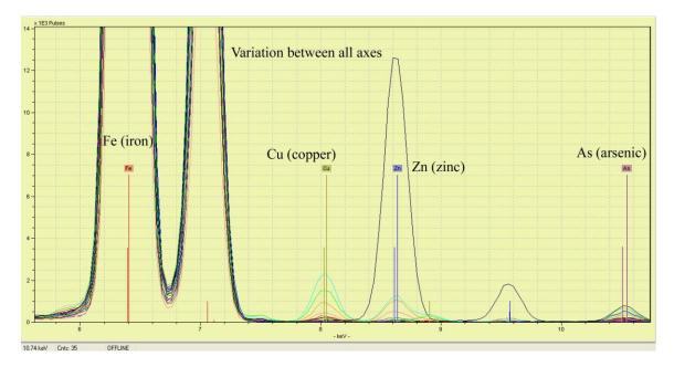
Figure 5:23 Variation visible in raw data pXRF spectroscopy of axes recovered from Fort Michilimackinac.
