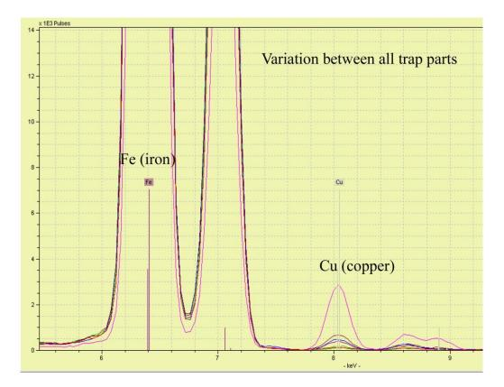
Figure 5:8 pXRF reading showing the variation between all trap parts analyzed in this sample.
