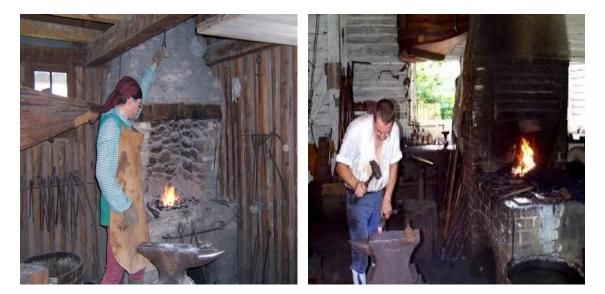
Figure 3:4 Examples of bellows positions. Reenactor from Fort Michilimackinac working with a side mounted bellows system (left) and a reenactor from Colonial Williamsburg working with a rear mounted bellows system (right). Photos taken by the author.
