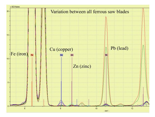
Figure 5:13 Raw data variation between ferrous saws. Note the presence of copper, zinc, and lead in various saw blades.
